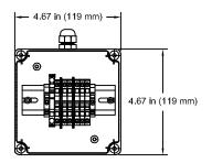
**CB - COMMUNICATION BOX** FULLY WIRED WITH CONTROL CABLE ENVIRONMENTAL RATING: IP67 (NEMA 4,4X,6)
