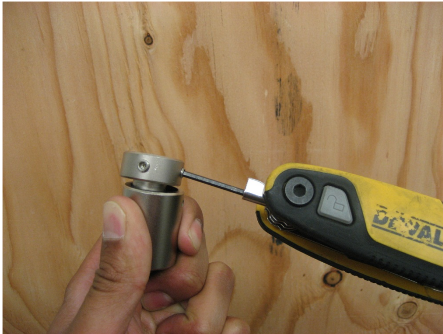
Figure 3 – Loosen 420DC coupling set screws
