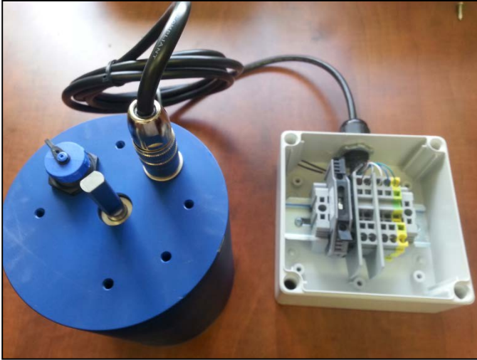
Figure 11 – Connect Actuator to Junction Box
