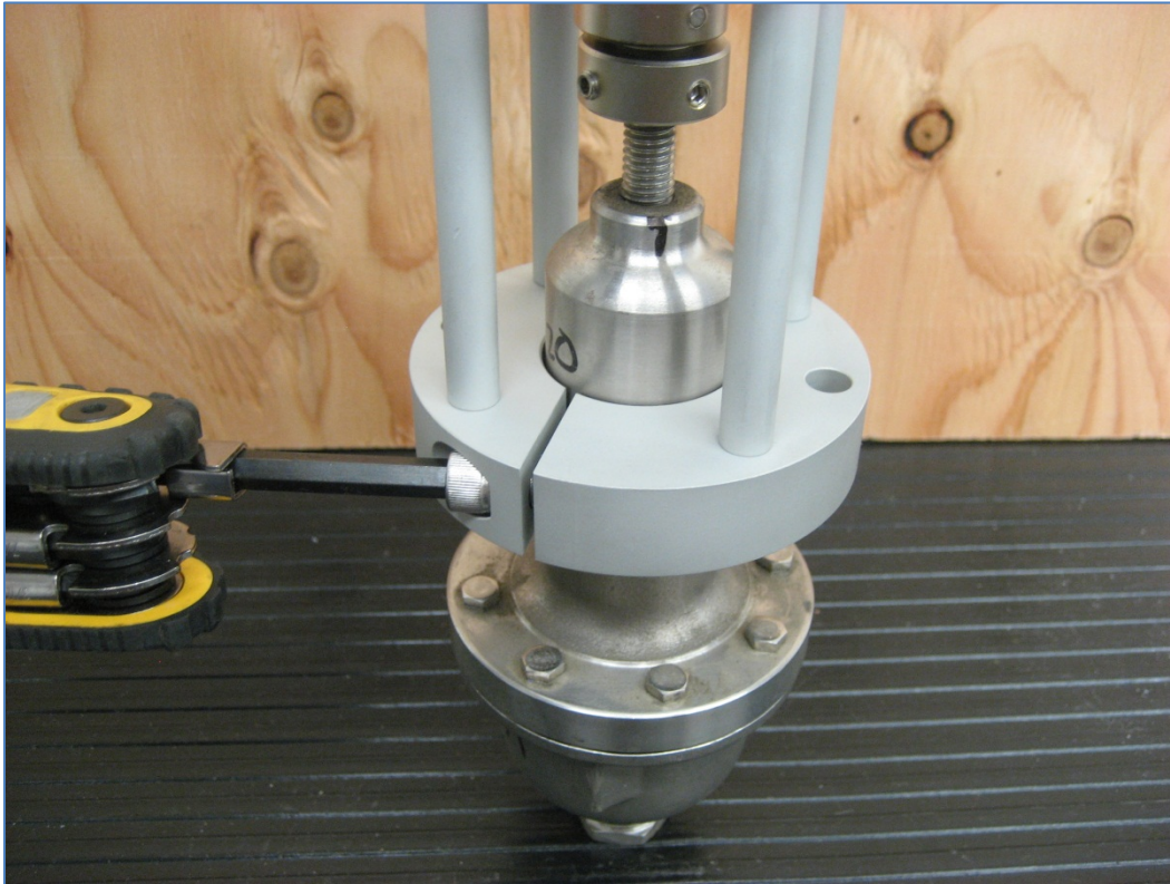
Figure 7 – Tighten spring casing set screws simultaneously
