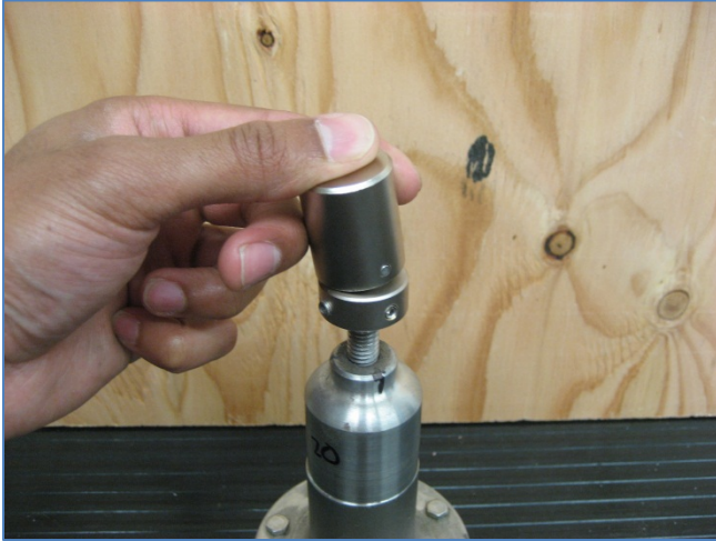
Figure 5 – Mount 420DC coupling to pilot adjustment screw
