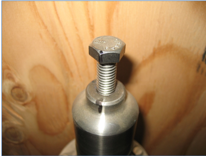
Figure 2 – Adjust pilot screw to minimum position
