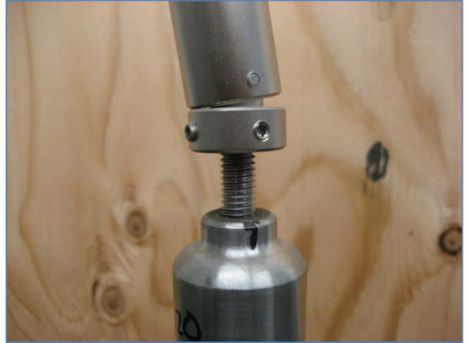
Figure 4 – Inspect assembly to ensure coupling sits flat
