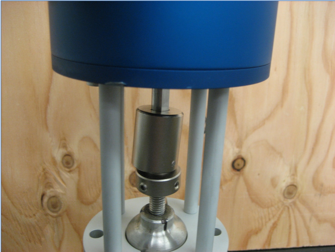
Figure 6 – Slip 420DC Actuator over pilot/coupling assembly and adjust orientation such that output shaft fits in top hole of coupling
